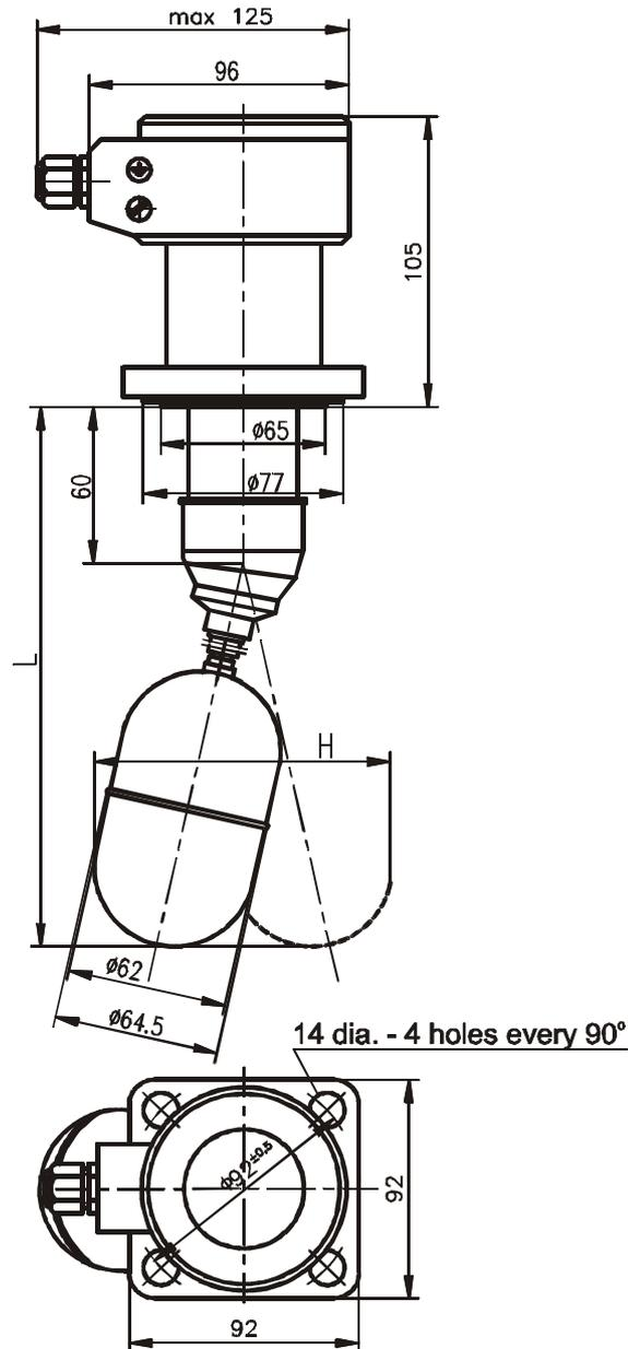
Dimension drawing of level switch type ERH-03-06
