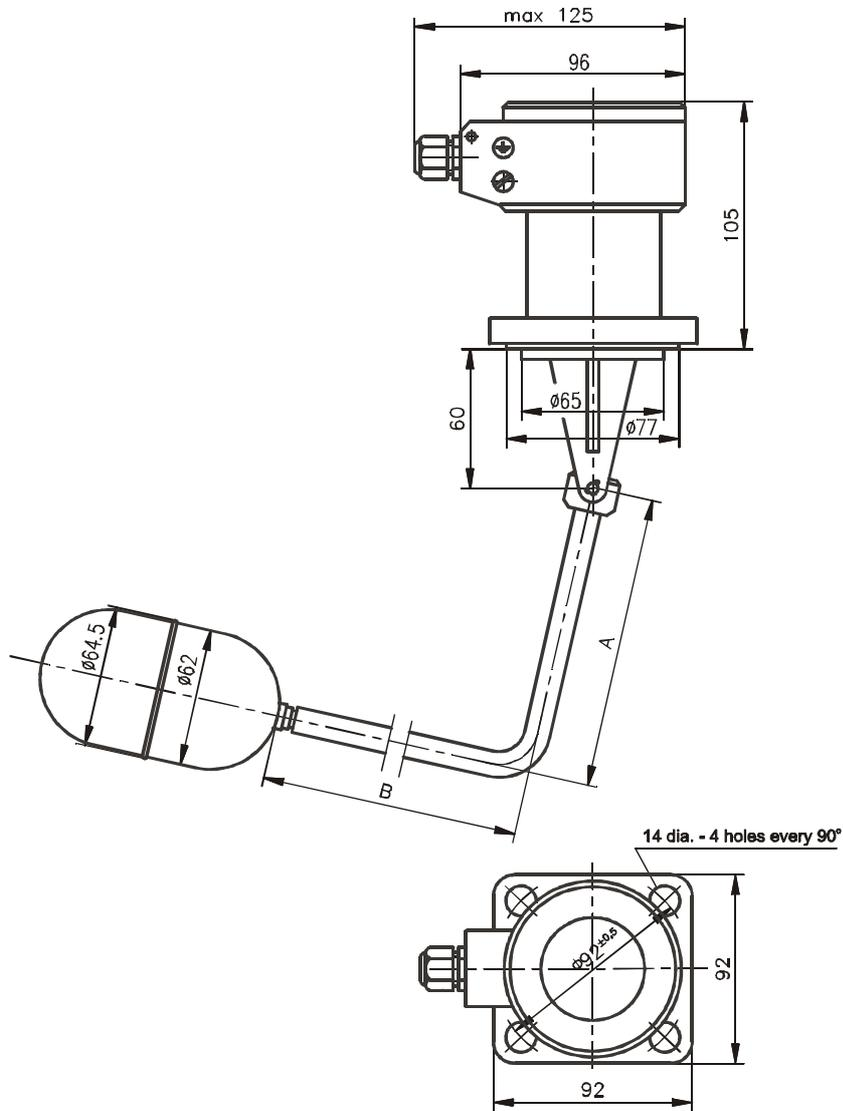
Dimension drawing of level switch type ERH-02-06
