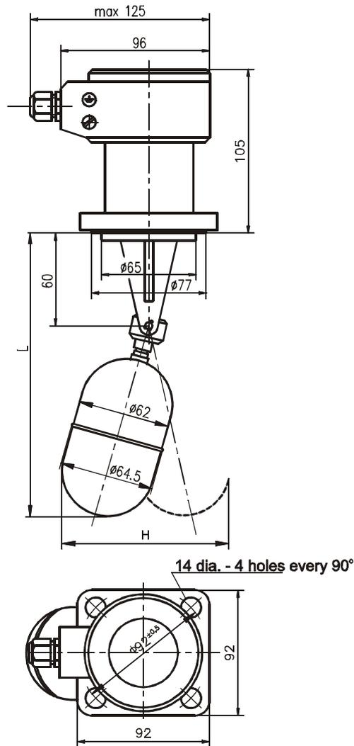
**Dimension drawing of level switch type ERH-01-06-4**
